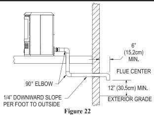
Minimum Exterior Grade Dimension - Single Flue, Horizontal Venting Below Floor
